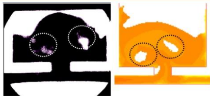
Evaluation of mold filling simulations using X-ray radiography
